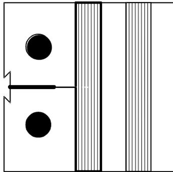
**Figure 7. Compact Tension Specimen Used for Fatigue Crack Growth Test**
