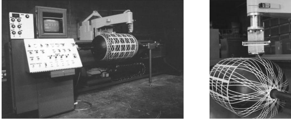
**Figure 1. Composite Filament Winding**
