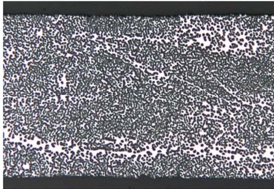
**Figure 4. Metallographic Section of MMC Filament Wound Cylinder**
