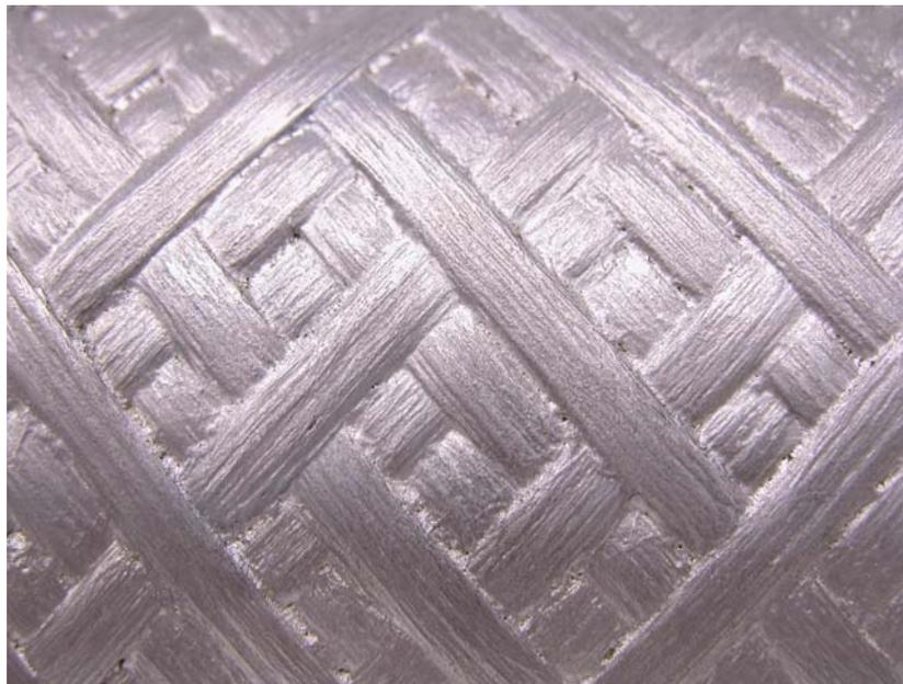
**Figure 3. MMC Filament Wound Helical Layer**
