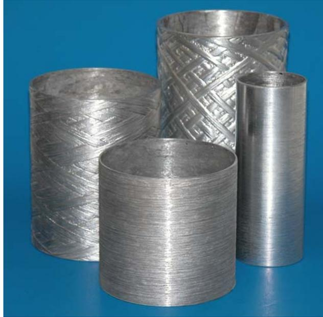
**Figure 2. MMC Filament Wound Cylinders**
