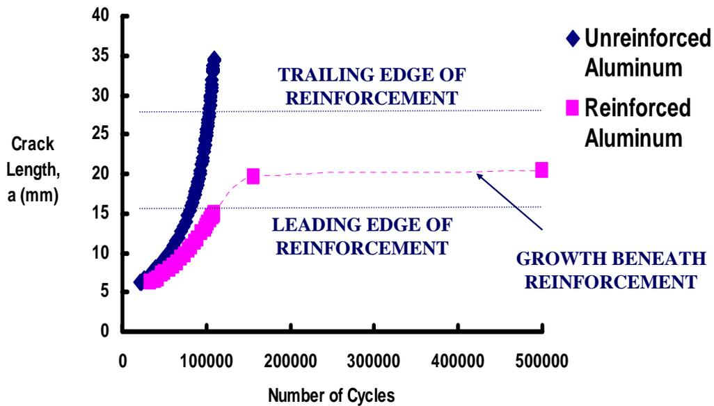
**Figure 8. Fatigue Crack Growth Data**
