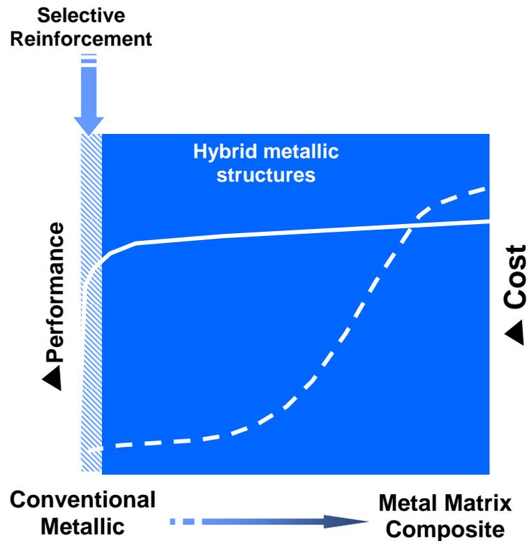
**Figure 6. Performance and Cost Trade-offs for Selectively Reinforced Structures**
