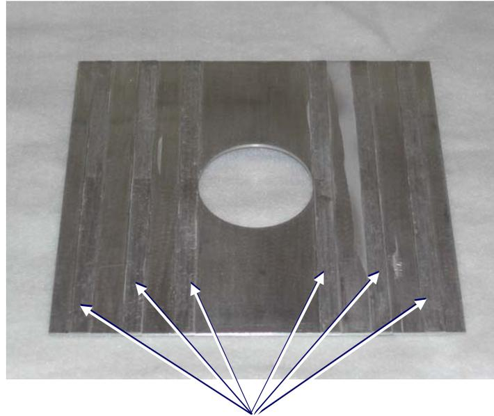
Longitudinal reinforcements adhesively bonded into slots machined in base aluminum structure
